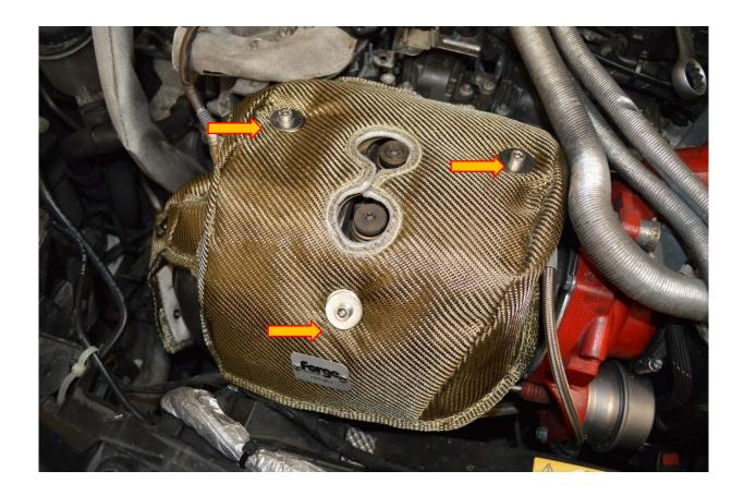
6. Using the two springs provided, wrap them around the down pipe and attach each end to the hooks on the turbo blanket.
